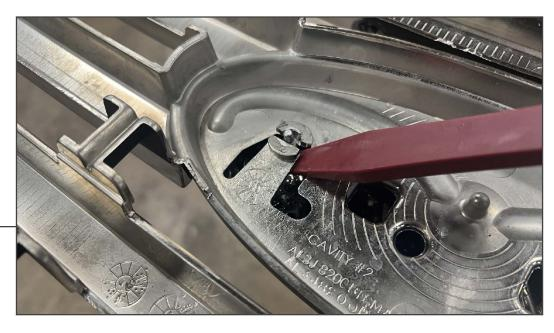
The grille emblem is double sided taped to the vehicle with posts fitted through the grille. Remove the (2) 10mm nuts from the rear of the emblem. Then, using a plastic pry tool, relieve tension from the posts while pulling/prying the emblem from the grille.
