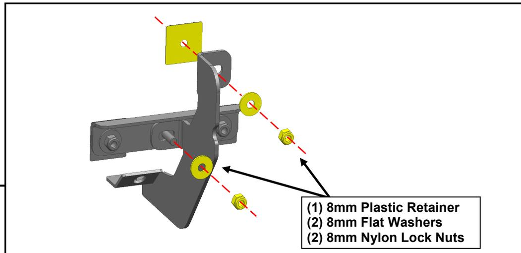
Loosely attach the (1) Passenger step bracket to the upper factory mounting stud and the (1) Passenger reinforcement bracket using (1) M8 plastic washer, (2) M8 flat washers, and (2) M8 nylon lock nuts.
