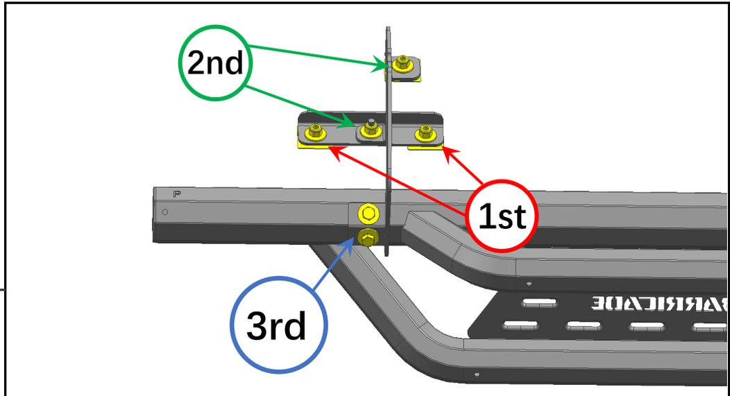
Tighten the mounting brackets to the vehicle. Adjust the side step to the desired angle, and tighten the M8 combo bolts to secure the step into place. See photo for tightening order visual.
