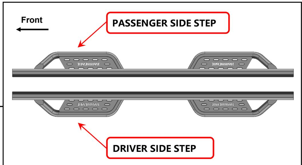
Identify each side step by identifier on the front. **Notice: "D" for Driver/Left Side; "P" for Passenger/Right Side.**
