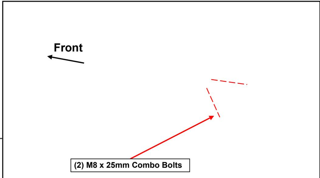
With all brackets loosely mounted to the vehicle, fit the side step onto the brackets, and loosely secure into place using (6) M8 x 25mm combo bolts.
