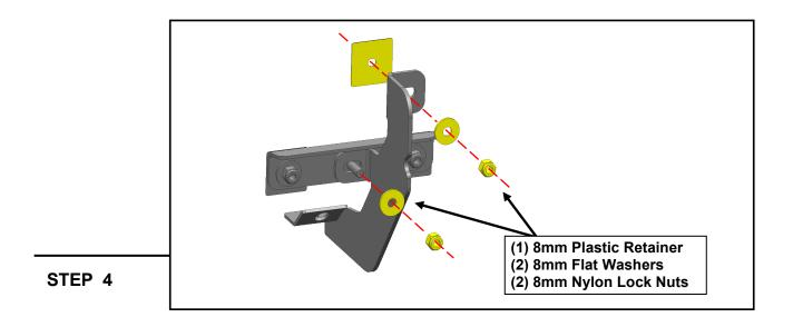
Loosely attach the (1) Passenger step bracket to the upper factory mounting stud and the (1) Passenger reinforcement bracket using (1) M8 plastic washer, (2) M8 flat washers, and (2) M8 nylon lock nuts.
