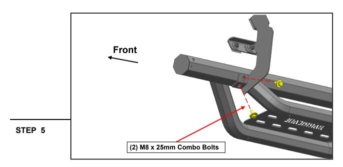
With all brackets loosely mounted to the vehicle, fit the drop step onto the brackets, and loosely secure into place using (4) M8 x 25mm combo bolts.
