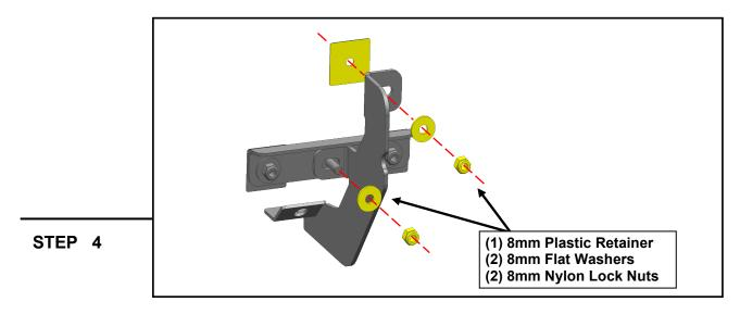
Loosely attach the (1) Passenger step bracket to the upper factory mounting stud and the (1) Passenger reinforcement bracket using (1) M8 plastic washer, (2) M8 flat washers, and (2) M8 nylon lock nuts.
