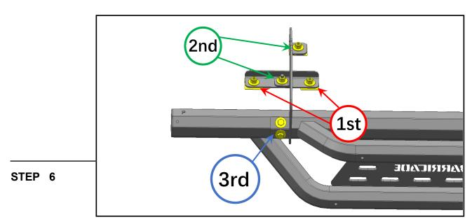
Tighten the mounting brackets to the vehicle. Adjust the running board to the desired angle, and tighten the M8 combo bolts to secure the step into place. See photo for tightening order visual.
