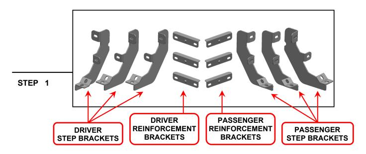
Mounting Brackets look very similar but are unique. Please identify each mounting bracket using the engraved location identifier. Notice: The Center brackets are the same as The Rear brackets. Both Reinforcement brackets are the same.
