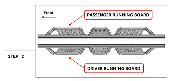
Identify each running board by identifier on the front. Notice: "D" for Driver/Left Side; "P" for Passenger/Right Side.
