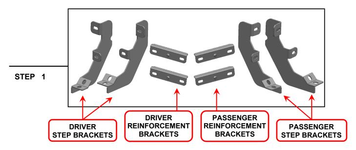
Mounting Brackets look very similar but are unique. Please identify each mounting bracket using the engraved location identifier. Notice: Both Reinforcement brackets are the same.
