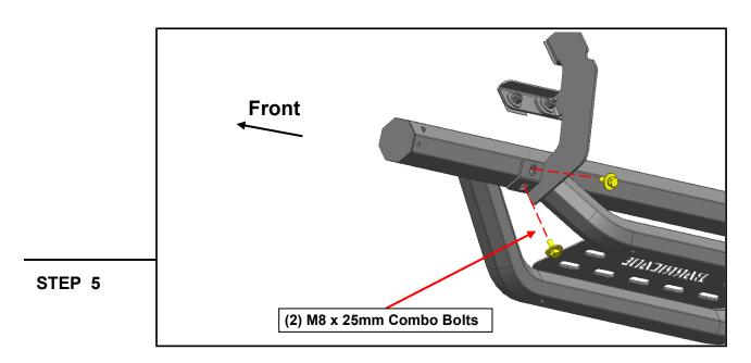
With all brackets loosely mounted to the vehicle, fit the drop step onto the brackets, and loosely secure into place using (4) M8 x 25mm combo bolts.
