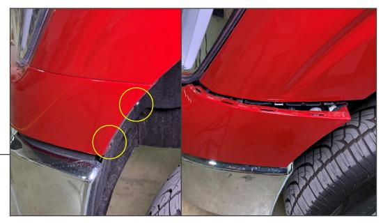
Above the front bumper, remove (2) 7mm bolts from inside the fender well securing the painted trim panel to the vehicle. Repeat this procedure to the opposite side.
