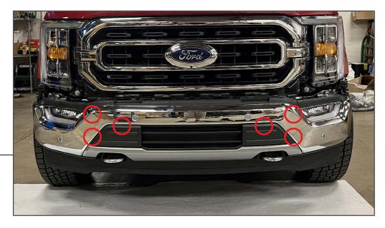
From under the vehicle, loosen the (6) 21mm nuts securing the bumper assembly to the vehicle. With a helper, remove all bumper mounting nuts and lift the bumper away from the vehicle and onto a soft workable surface.
