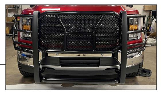
Adjust the grille guard to best fit the vehicle. Loosening & tightening the bumper/grille guard to achieve proper fitment may be necessary.
