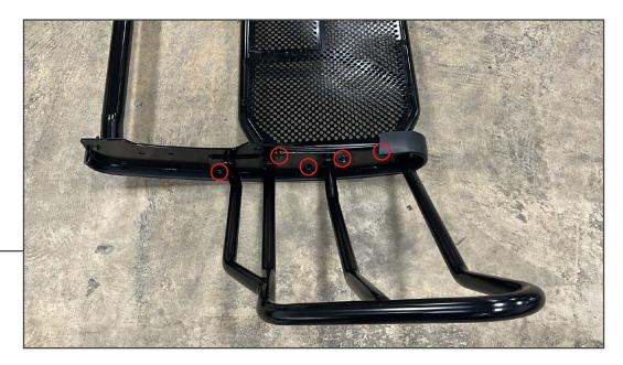
Fit the center grille guard panel in between the LH and RH bumper panels. Then, align each headlight guard to the center grille guard panel and the bumper panels. Once aligned, loosely secure the panels together using (10) M8 x 35mm bolts, (20) M8 flat washers [24mm OD], and (10) M8 lock nuts.
