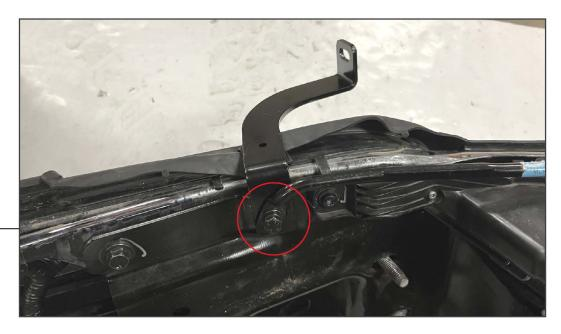
Fit the included upper mounting bracket to the bumper, and secure into place using (1) M8 x 50mm bolt, (1) M8 lock washer, and (1) M8 flat washer [22mm OD]. Repeat this step for the opposite side of the bumper.
