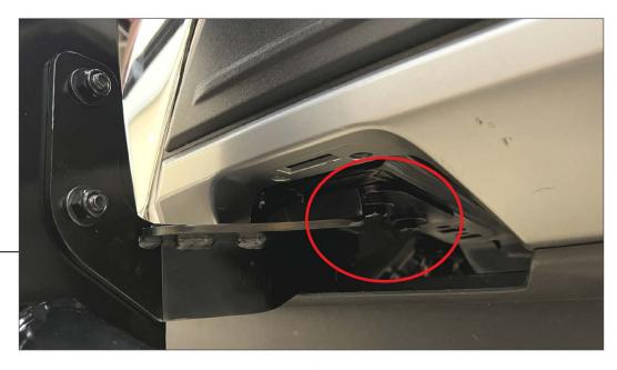
Re-install the bumper to the vehicle reusing the original (6) 21mm nuts. Re-install the upper painted trim panel using the original (4) 7mm screws. Plug the front bumper harness into the vehicle chassis harness.
