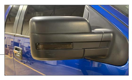
Test the light by turning on the respective turn signal. Once the light is confirmed working, follow steps 1-3 in reverse order to re-assemble the mirror assembly.
