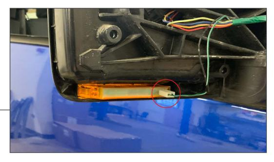
Remove the factory wiring harness from the light.
