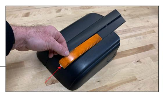
Remove the original orange reflector from the outer mirror shell. Pry on the outer edge to unclip it from the housing.
