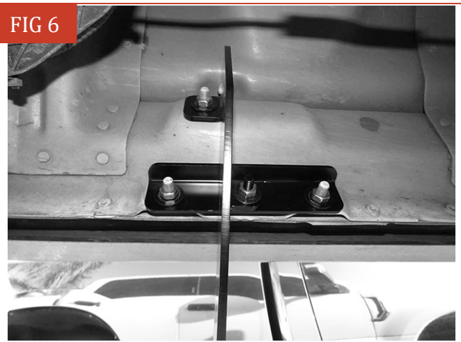
(Fig 6) Example of the Mounting Bracket attached to the upper mounting stud and Support Bracket
