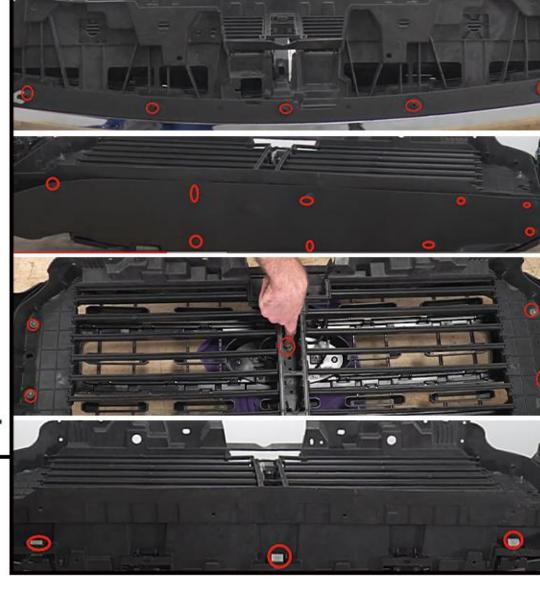
Remove two 7-millimeter bolts on each side with a 7-millimeter socket and pop out a bunch of clips to remove the lower trim.
