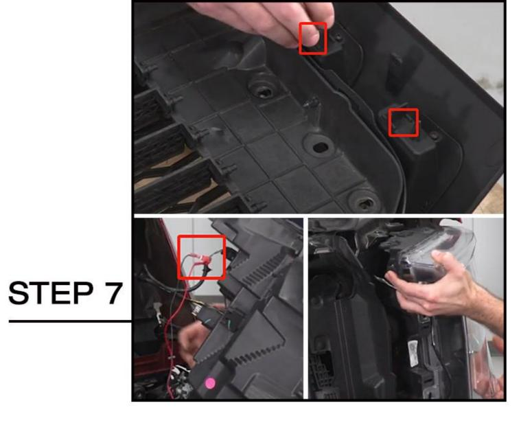
Install clips onto both sides. Plug the red wire of the grille into the positive wire of the headlight and black to the negative wire. Follow the step 5 in reverse order to reinstall the headlight.
