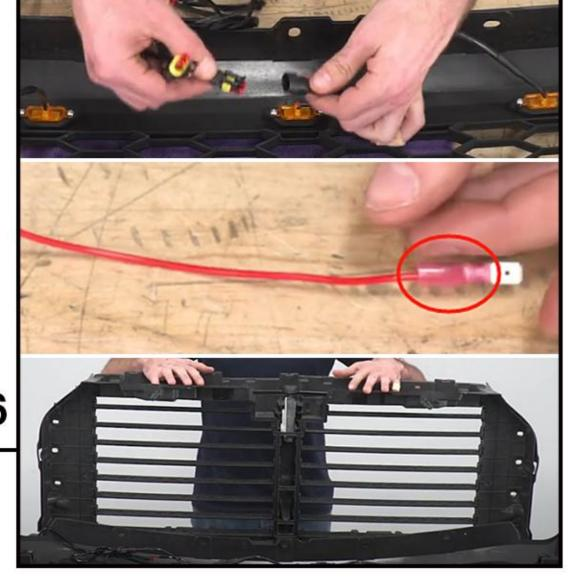
Connect each amber light to the wiring harness. Crimp the male spade connectors onto the positive and negative. Follow the step 4 in reverse order to reinstall shutter assembly onto the new grille.
