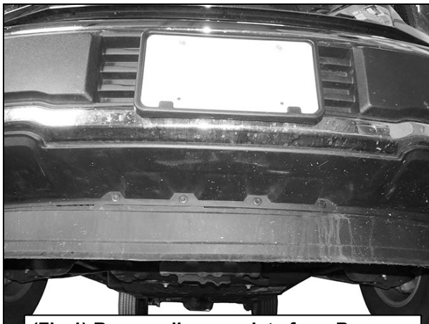
(Fig 1) Remove license plate from Bumper
