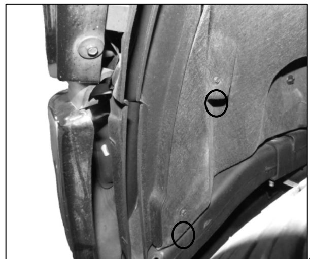
(Fig 2) Remove the plastic bumper pad from the front of the Bumper
