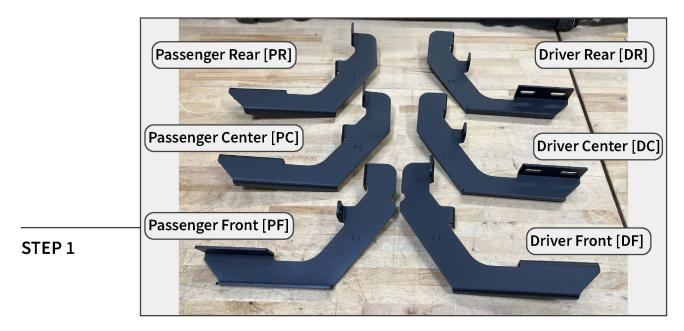
Identify the running board mounting brackets using the diagram above. The front mounting brackets are different from the center/rear brackets.
