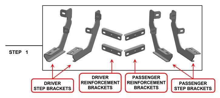
Mounting Brackets look very similar but are unique. Please identify each mounting bracket using the engraved location identifier. Both Reinforcement brackets are the same.
