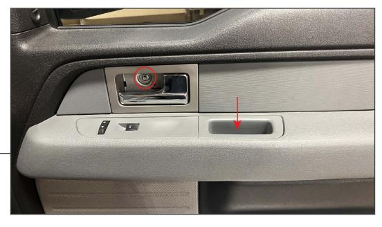
It is recommended to lower the vehicle window before disassembly. Open the vehicle door.
