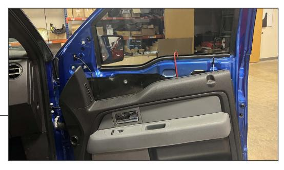
Lift the door panel upwards to unhook the panel from the door. Disconnect the door release cable from the door release handle, or carefully hang the door panel.
