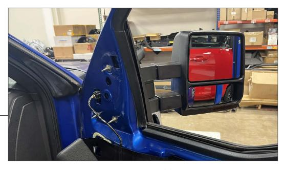
Fit the new mirror to the vehicle, and secure using the included (3) 10mm nuts.
