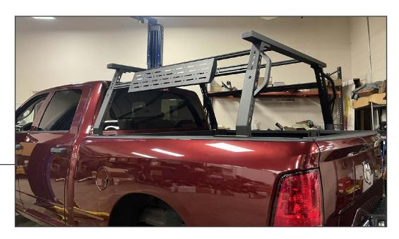
Ensure all bed rack hardware is fully secure.
