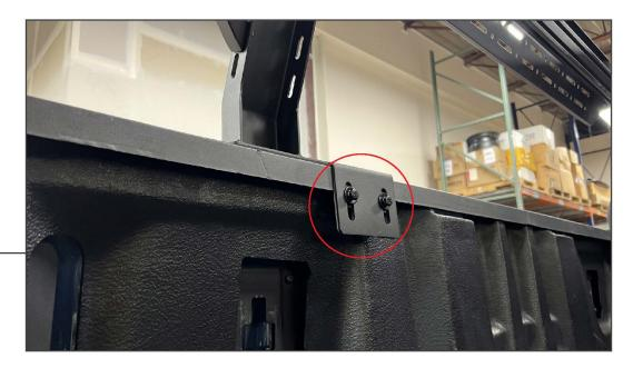
With assistance, lift the bed rack onto the vehicle bed rails. Adjust the bed rack width as necessary using the cross bar adjustment slots. Tighten the rack to the bed rails following the applicable procedure in Step 6. Tighten all mounting hardware evenly, then tighten the cross bar adjustment bolts.
