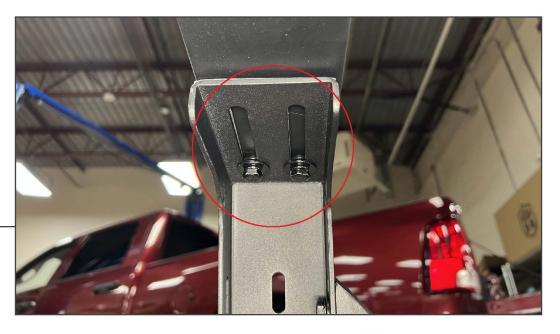
Loosely secure the assembled mounting bracket to the cross bar using (2) M8 x 25mm combo bolts into the threaded inserts in the cross bar. The mounting brackets will adjust to the vehicle bed rail utilizing the slotted holes in the mounting bracket.
