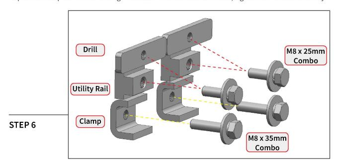
Identify the bed rack mounting hardware. Depending on the vehicle/application, different mounting hardware will be used.
