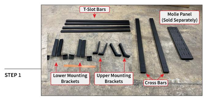
Lay out and identify all bed rack components.
