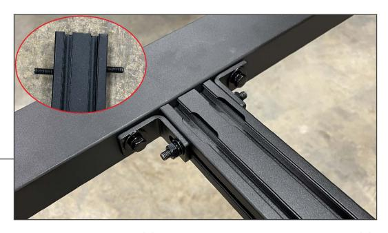
Fit (2) M8 square head studs onto each side of (2) remaining T-Slot bars. Then, fit the included (2) "L" brackets onto the studs. Loosely secure the "L" brackets using (2) M8 flat washers, (2) M8 lock washers, and (2) M8 nuts.
