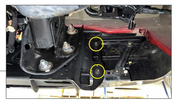
The bed corner step can only be installed on the LH (Driver's) side of the vehicle.
