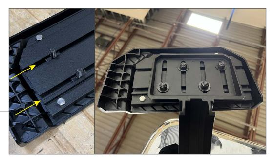
Slide (2) T-Studs into each row on the bottom of the step pad. Then, position the studs through the step hinge assembly pad. Secure the step pad to the hinge assembly using (4) M8 flat washers and (4) M8 lock nuts. Tighten evenly until secure.
