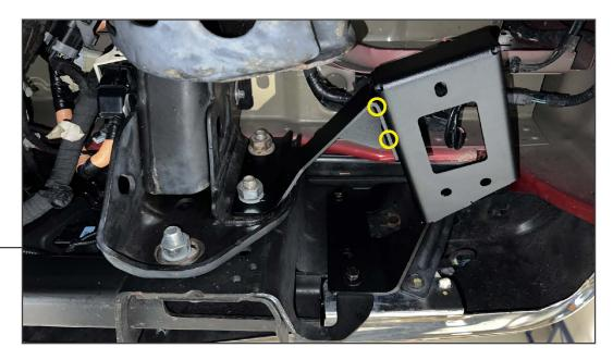
Secure the bumper and frame mounting brackets together using (2) M8 combo bolts.
