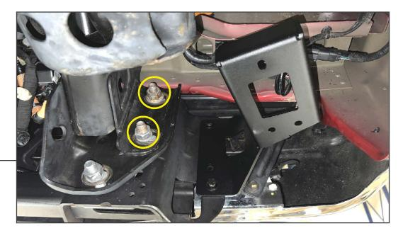
Loosen and remove the (2) 21mm nuts securing the bumper to the frame.
