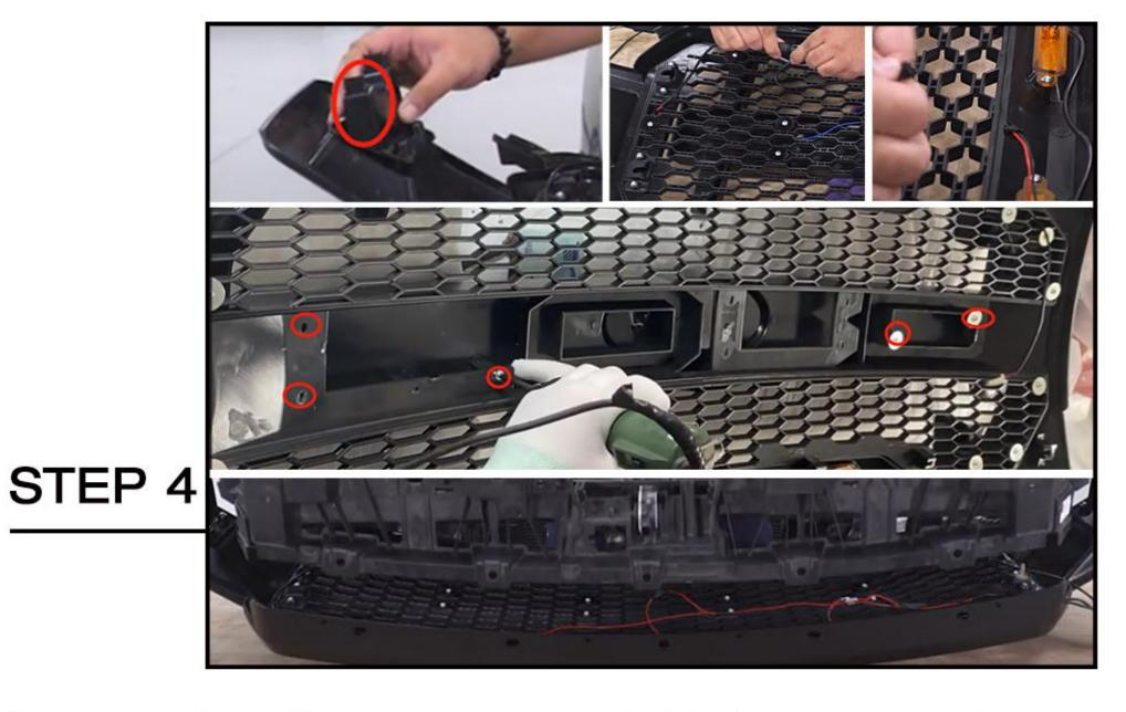
Install the headlight clip post on both side, connect the amber lights with wiring harness. Loosen 5 screws to remove the horizontal bar. Remove the "Ford" emblem from the original grille and install it on the horizontal bar, tighten 5 screws again to install the horizontal bar. After that, follow the step 3 in reverse order to assemle the inner grille with the outer grille.
