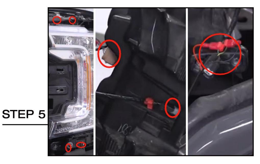
Remove 4 bolts to remove the headlight, then disconnect the harness. Crimp the male spade connectors onto the positive and negative wiring for the 3 amber lights on the grille, place T-taps on the positive and negative wires of the headlights separately, and plug them into the
