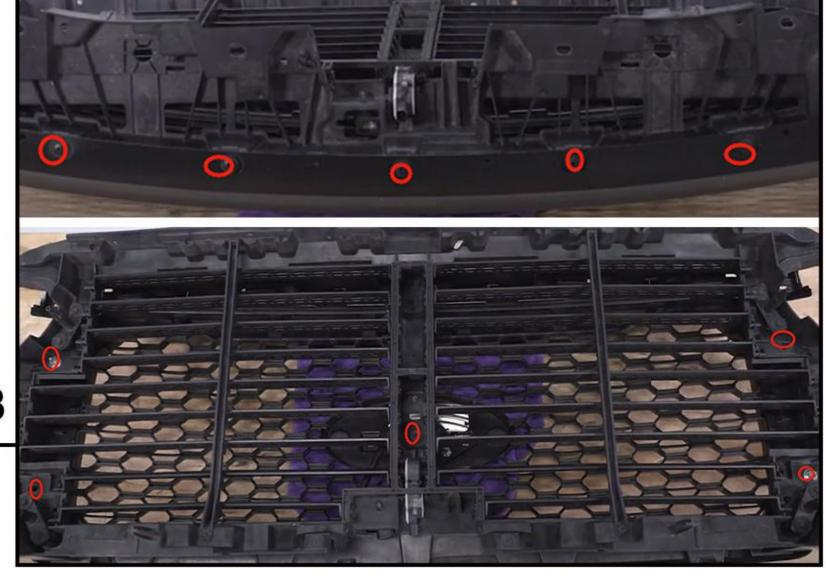
Open the hood, remove all the push pins to remove the radiator cover, then remove the 4 bolts at the top of the grille.
