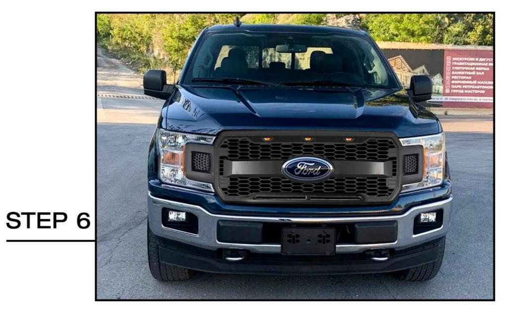
After connecting the wires, follow the step 5 in reverse order to reinstall the headlights. Put the new grille back on the car and follow the step 1 & 2 in reverse order to install the new grille.
