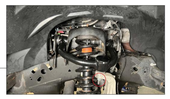
Re-assemble the vehicle suspension components following steps 1-6 in reverse order. Secure the upper ball joint to the vehicle steering knuckle using the included 19mm nut.
