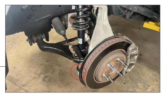
Remove (1) 21mm nut from the tie rod end. Strike the steering knuckle with a hammer to dislodge the tie rod end from the knuckle.
