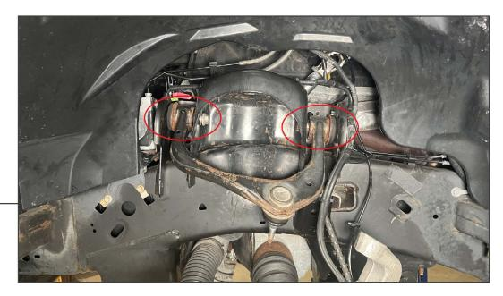
Remove the (2) control arm bolts from the vehicle. Then, use a pry bar to remove the control arm from the vehicle frame. Set the control arm aside.
