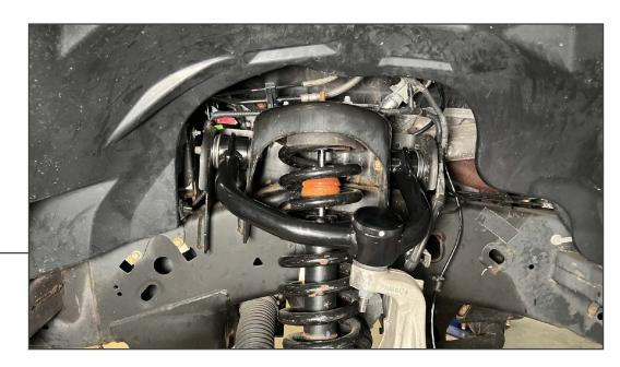
With the vehicle suspension loaded, torque the upper control arm bolts evenly to 122 ft. lbs.
