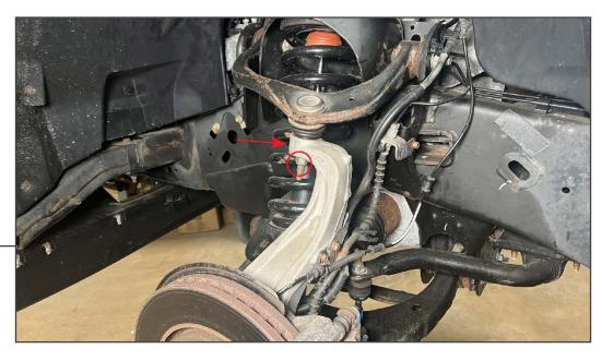
Loosen the 18mm nut securing the upper ball joint to the knuckle. Using a hammer, strike the steering knuckle to separate the ball joint from the knuckle. Remove the nut to separate the control arm from the knuckle. This will allow additional space when removing the strut assembly from the vehicle.
