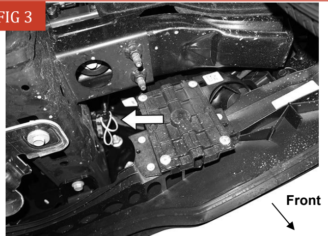
(Fig 3) Locate and unplug main harness plug on passenger/right side of bumper (arrow)
