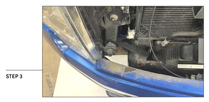
Loosely mount the appropriate mounting bracket to the grille bumper using the original T-30 Torx screw on each side of the vehicle.
