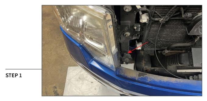
Open the vehicle hood. Locate the grille bumper, and remove (1) T-30 Torx screw.
