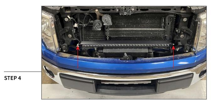
Fit the LED light bar in-between the mounting brackets, and loosely secure into place using (1) M8 x 20mm Allen bolt, (1) M8 lock washer, and (1) M8 flat washer per side.
