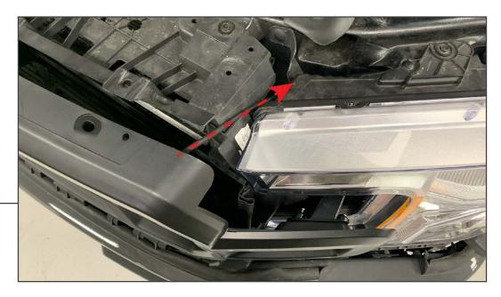
Position the grille to the vehicle, allowing the wiring to route towards the LH side headlight.
