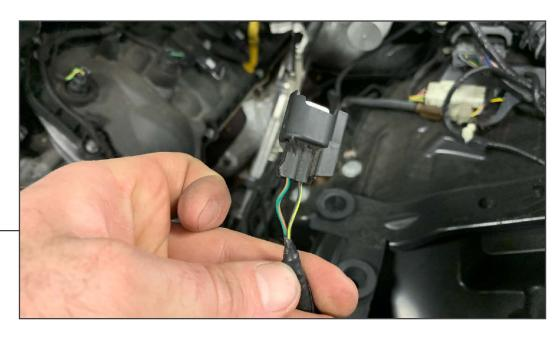
Amber Parking Lamp Wiring Harness: Using the supplied scotchlok connectors, connect the vehicle parking lamp wiring to the LED light harness using the diagram below. After wiring the LED lights, re-install the headlight using OEM hardware.
