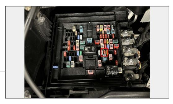
**DRL & Turn Signal LED Lights Wiring (cont.):** Install the included fuse tap to the red wire lead, and the included ring terminal to the black wire lead. Fit the fuse tap into the vehicle fuse box replacing fuse # 36. Then, route the wiring out of the fuse box and re-install the lid. Secure the ground ring terminal to a clean suitable grounding point.
