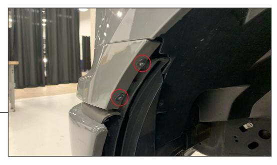
Use a 7mm socket to remove the (4) screws ((2) on each side) securing the front fascia to the vehicle.
