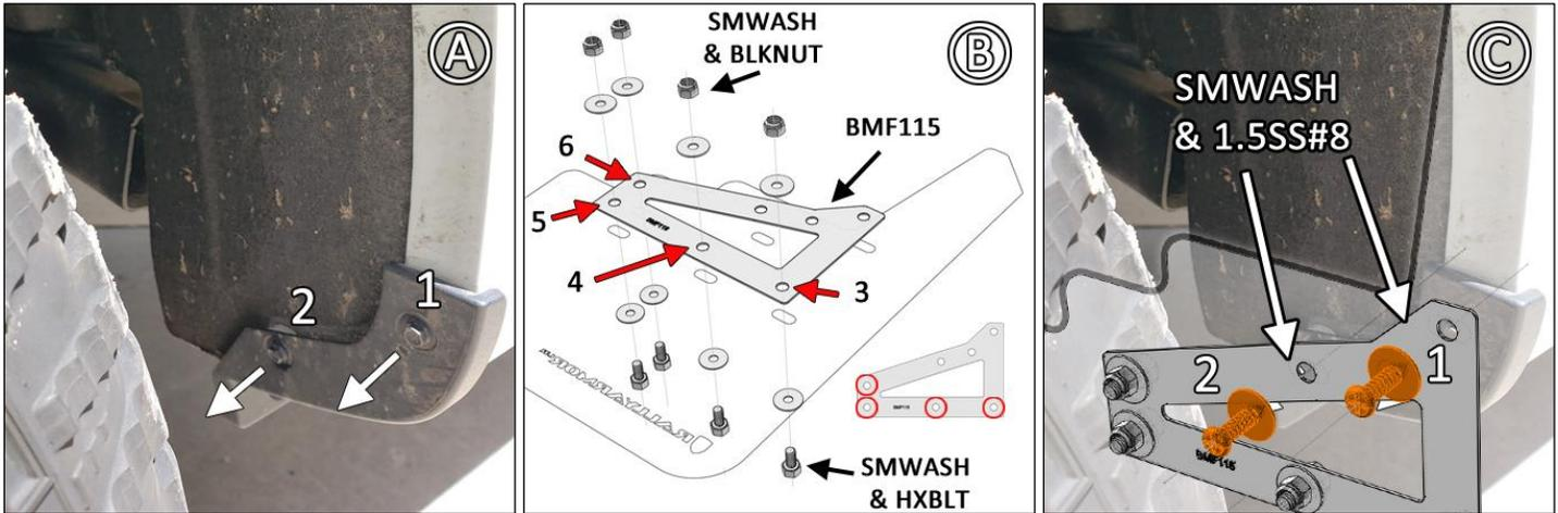
**FIGURE D** Align flap to even ground, then secure top portion of flap.
