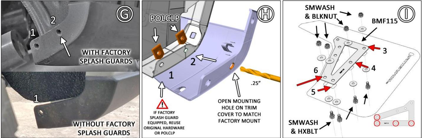
**FIGURE J** Install SMWASH & 1SS into mounts 1 & 2. If equipped with splash guards, reuse factory hardware.
