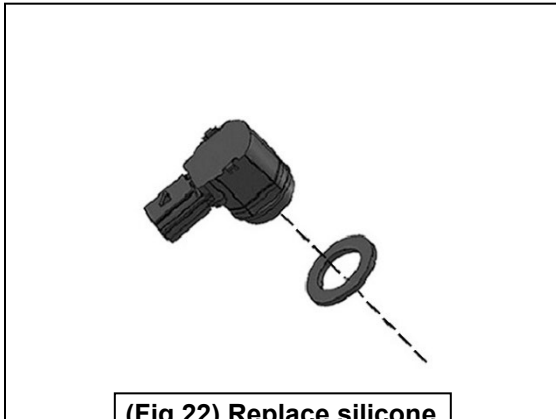
(Fig 22) Replace silicone seal with large Seal
