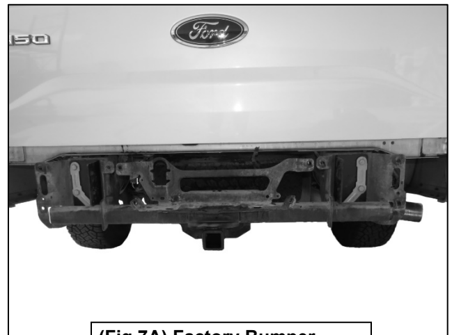
(Fig 7A) Factory Bumper removed (with receiver hitch)
