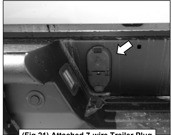
(Fig 21) Attached 7-wire Trailer Plug
