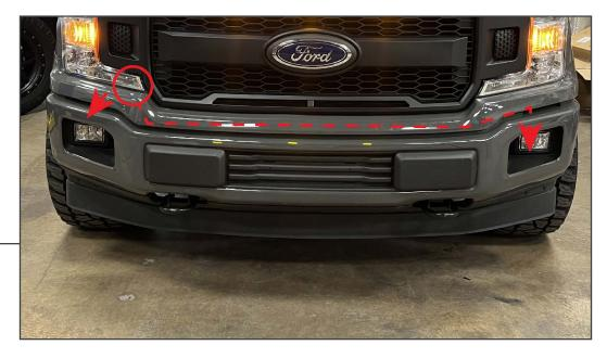
From under the vehicle, locate the fog light wiring harness routing from the passenger side of the vehicle towards the driver side. Unplug the fog light harness connector along the passenger side frame rail. Using a panel removal tool, dislodge the harness retainers from the vehicle and remove the harness from the vehicle.
