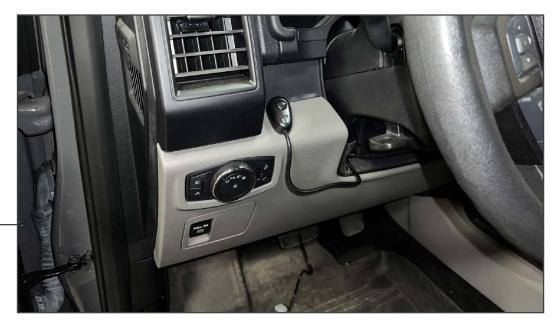
Using the included double sided tape attached to the switch, fit the switch to the desired position on the dashboard. Route the harness towards the vehicle firewall grommet, and plug the connectors together. Ensure the harness is secure away from the steering/pedal assemblies.
