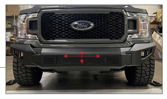
With a helper, carefully fit the bumper to the vehicle frame rails, and secure using the original bumper mounting nuts. Adjust until the bumper is evenly fitted to the vehicle, and tighten the hardware until the bumper is secure.
