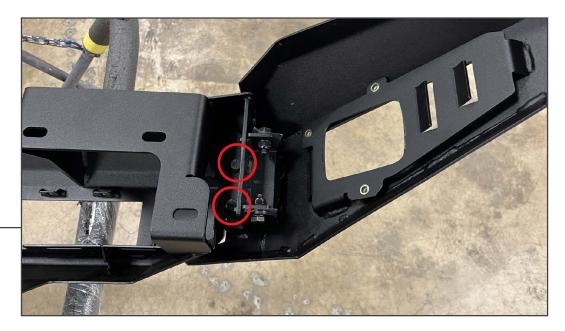
Place the new bumper on a workable surface for assembly. Fully fold the outer corners of the bumper, and secure the corners using (4) M10 x 30mm bolts, (4) M10 lock washers, and (4) M10 flat washers.
