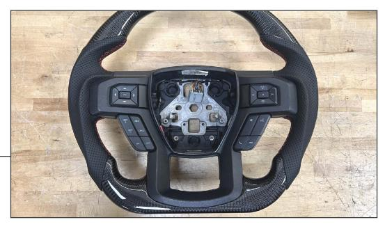
Align the steering wheel control assembly to the new steering wheel, and route the harness into place. Once the harness is properly routed, press the steering wheel control assembly fully into place. Work around the perimeter to ensure an even fit.
