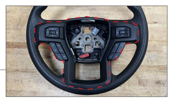
Using a plastic pry tool, work around the perimeter of the steering wheel controls and lower trim panel. This assembly is secured in some areas using large plastic dowels in the steering wheel foam. These dowels can be difficult to remove and sometimes require additional pressure/force to dislodge.
