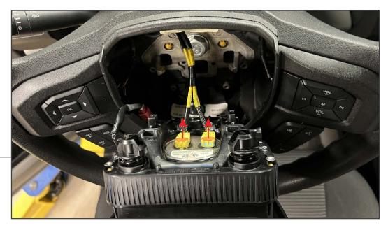
Using a small pry tool, lift the orange connector locks away from each yellow connector. With the orange locks lifted, the connector will lift out of place. Gently use the pry tools to lift the connector upwards if necessary.
