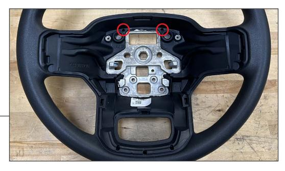
Lift the steering wheel control and lower trim panel assembly away, and dislodge the harness from the steering wheel. Use a small pry tool to dislodge the (2) retaining push clips.
