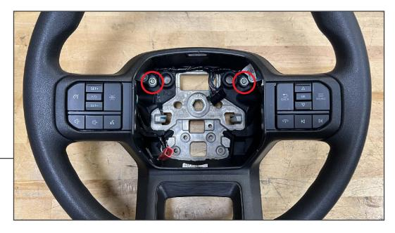
Begin to disassemble the steering wheel by removing the (2) T-20 Torx screws.
