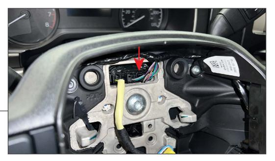
Unplug the steering wheel controls connector by pressing the tab and pulling the connector away.
