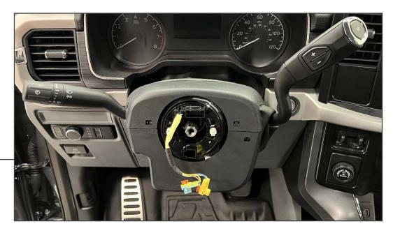
Lift the steering wheel from the vehicle. While removing the steering wheel, carefully route the clockspring wiring harness out of the steering wheel. Ensure the clockspring remains in the original position. If the clockspring moves slightly during steering wheel removal, gently move back to the original starting position.
