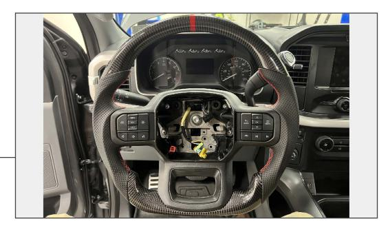
Align the steering wheel to the vehicle, and route the clockspring harness through the steering wheel. Fit the steering wheel to the steering column and secure into place using the original T-50 Torx bolt.
