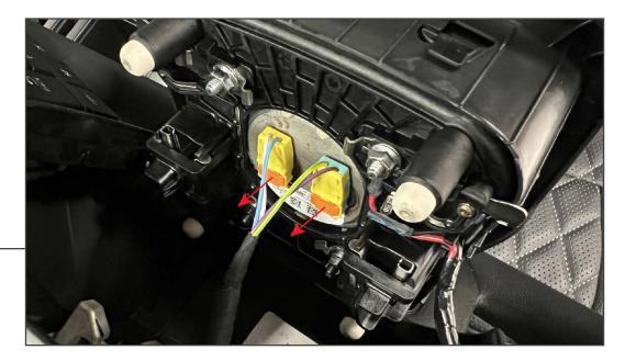
Using a small pry tool, lift the orange connector locks away from each yellow connector. With the orange locks lifted, the connector will lift out of place. Gently use the pry tools to lift the connector upwards if necessary.
