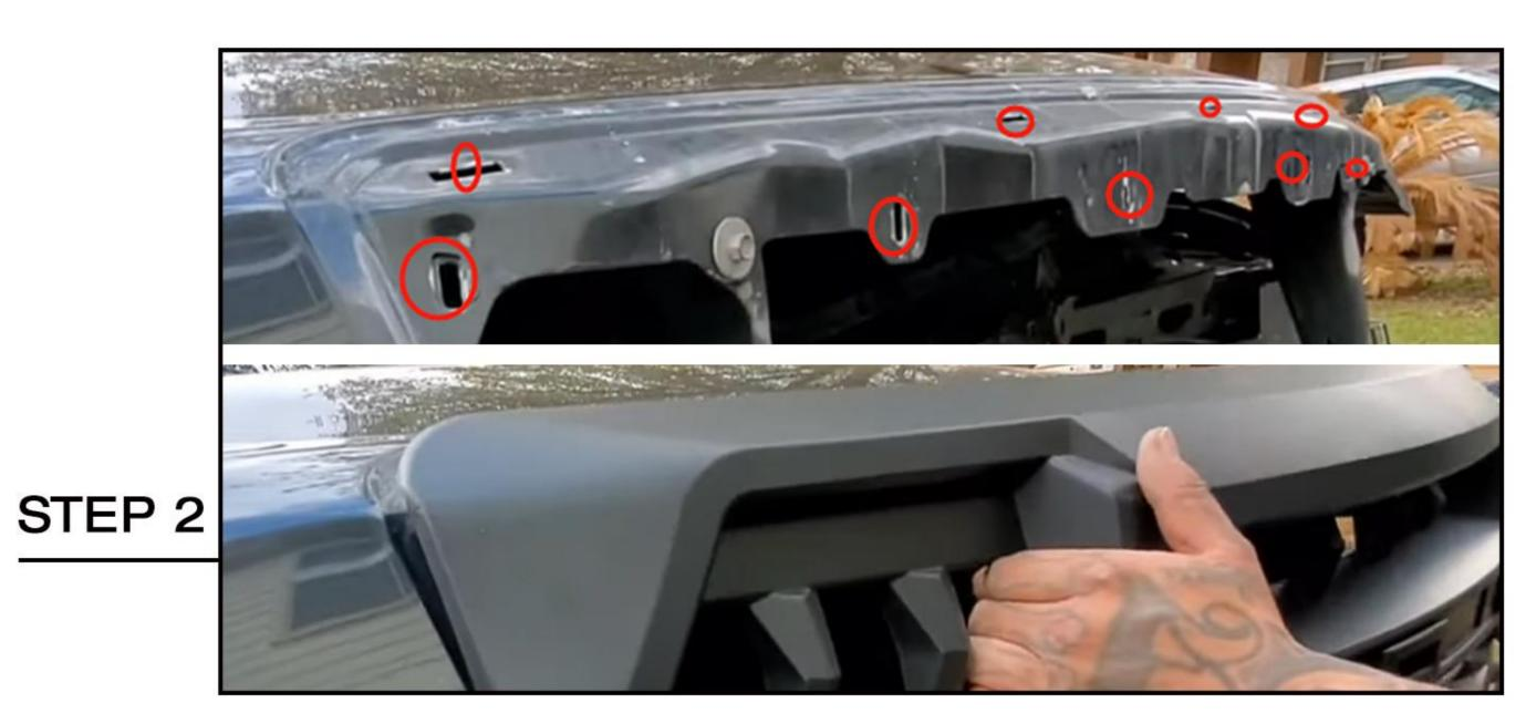
Pop the clips right up in the holes that was circled in the picture and screw the new grille.
