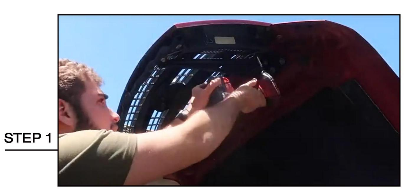
Remove the eight screws onto the front hood and six screws holding it down to the actual face of the hood.
