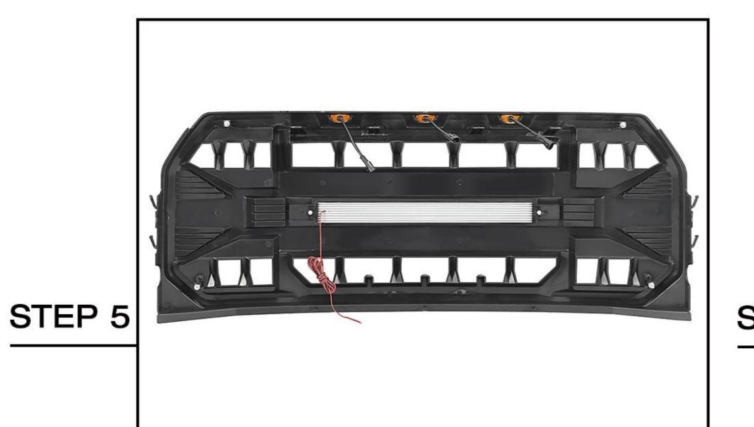
Amber lights wiring: First connect each amber light to the wiring harness, then connect the red wire to ACC, and the black wire to the negative of battery.
