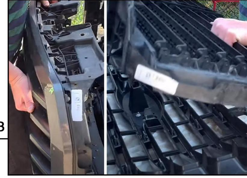
Remove all the little pushpins to remove this shroud piece.
