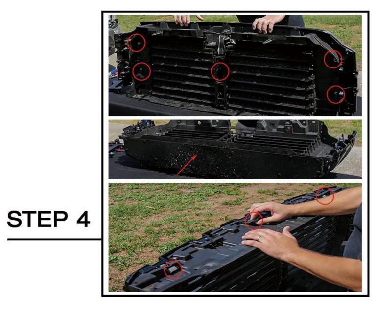
Remove the 4 screws holding the trim piece on the left
