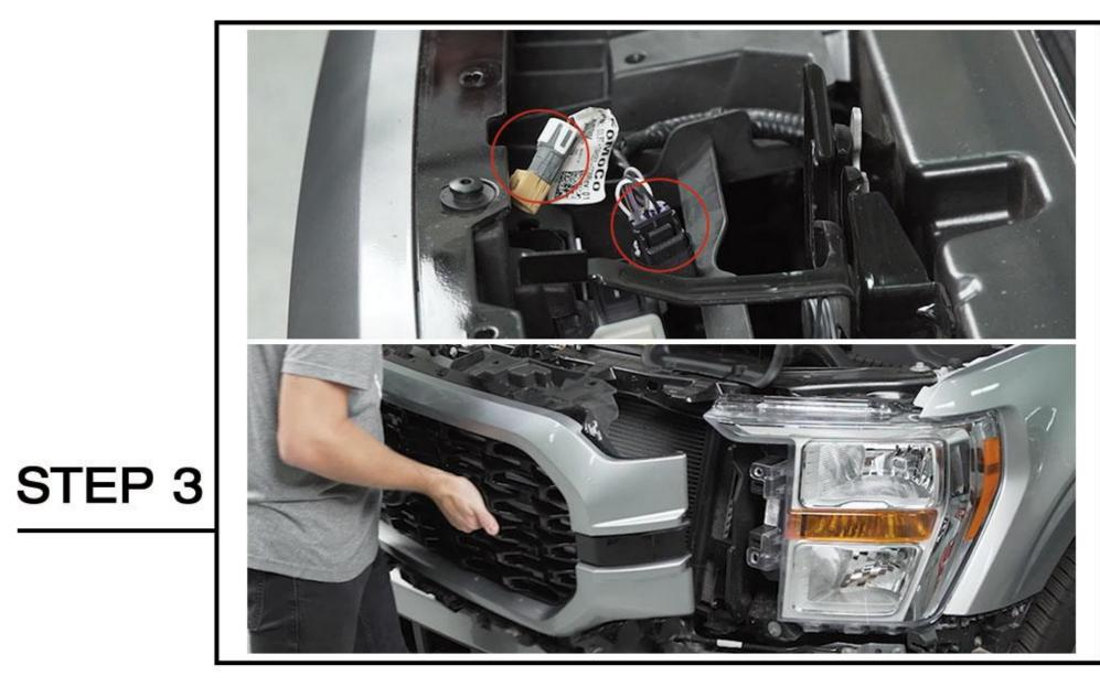
Unplug the 2 wire harnesses and pull the whole grille assembly from the truck.
