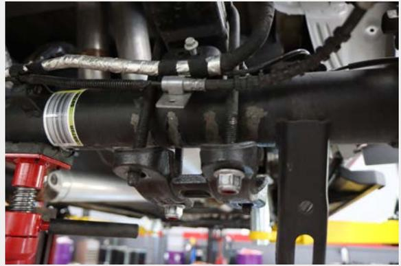
Figure 1: U-bolt Removal
