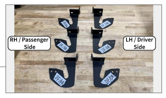
Identify the side steps mounting brackets using the diagram above. The LH and RH mounting brackets are different.
