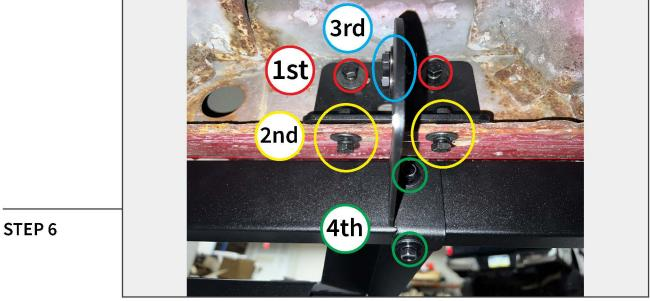
Adjust the side step to best fit the vehicle, then tighten the mounting hardware following the diagram above.
