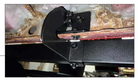
With a helper, align the side step to the previously mounted step brackets. Loosely secure the side step to the step brackets using (2) M8 x 25mm combo bolts per bracket.
