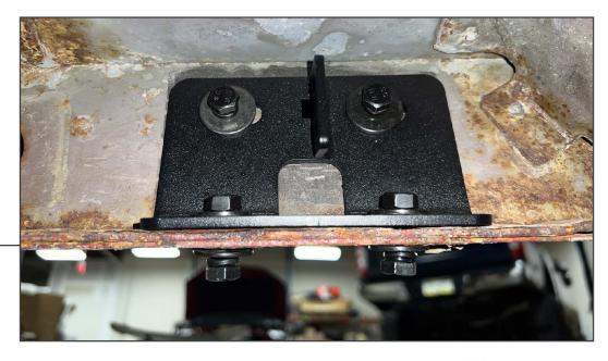
Loosely secure the rectangular brackets to the bottom of the rocker panel using (2) M8 x 30mm bolts, (4) M8 flat washers [22mm OD], and (2) M8 lock nuts per bracket.
