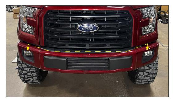
From under the vehicle, locate the fog light wiring harness routing from the passenger side of the vehicle towards the driver side. Unplug the fog lights from the harness. Using a panel removal tool, dislodge the harness retainers from the vehicle bumper.
