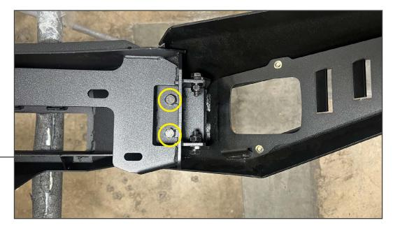
Un-fold the bumper end caps. Then, secure the end caps using (2) M10 x 30mm bolts, (2) M10 lock washers, and (2) M10 flat washers per end cap.
