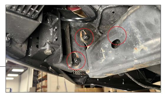
With a helper, lift the new bumper to the vehicle, and secure into place using (6) M12 x 35mm bolts, (6) M12 lock washers, (12) M12 flat washers, and (6) M12 nuts. Adjust the bumper to best fit the vehicle, and then tighten all hardware to fully secure the bumper into place.
