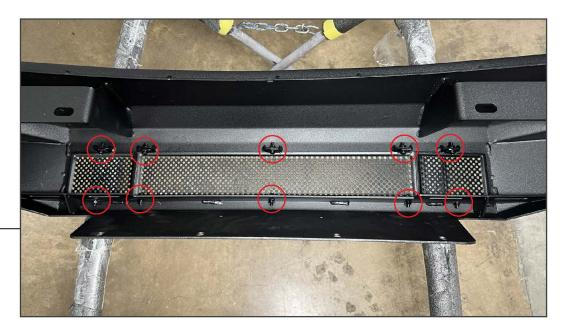
Secure the LH, RH, and Center mesh panels to the bumper using (10) M6 x 20mm combo Allen bolts and (10) M6 flange nuts.
