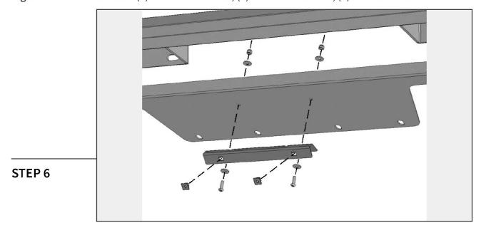
If desired, secure the front license plate mounting bracket to the bottom of the bumper using (2) M6 x 20mm Allen bolts, (4) M6 flat washers, and (2) M6 lock nuts. Then, fit the (2) square plastic screw retainers into the square holes in the bracket.
