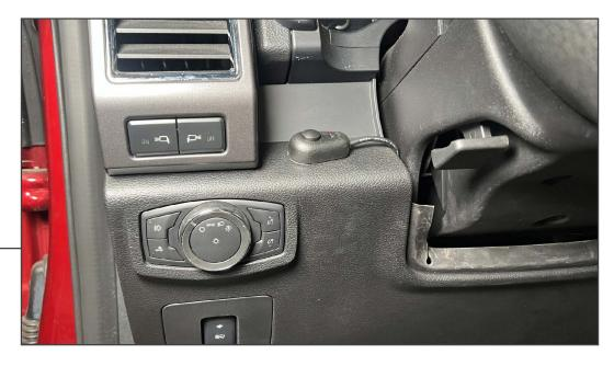
Using the included double sided tape attached to the switch, fit the switch to the desired position on the dashboard. Route the harness towards the vehicle firewall grommet, and plug the connectors together. Ensure the harness is secure away from the steering/pedal assemblies.
