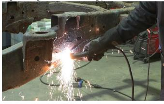
Grind down the frame free of rust and debris, revealing bare metal.
