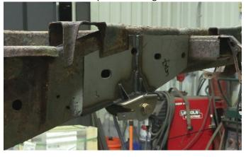
Following proper welding procedures, tac weld the frame section to the frame. Confirm its fitment, and weld the part on fully. Weld 100% around all edges.
