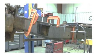
Following proper welding procedures, tac weld your front frame section onto the frame before welding it on fully. Weld 100% around all edges.
