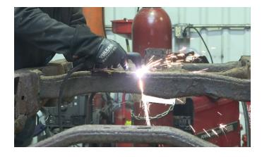
Clean and grind the work area free of rust and debris, revealing bare metal.
