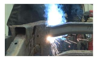
Place the included shock mounts onto the outside ends of the crossmember while leaving about a 1/8" space from the edge, followed by welding them into place. Note: The shock mounts are driver and passenger specific. When pushed into place, they should tilt away from the frame.
