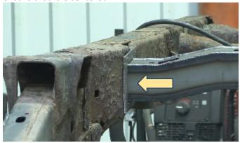
Tac weld the plates into place before fully welding the inside and outside edges to the crossmember and frame rails.
