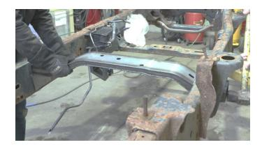
Slide the inner plates to where they sit against the inner side of the frame rail.
