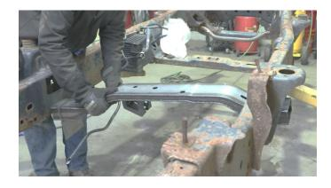
Then, slide your crossmember into place, one side at a time. Tap it into place using a hammer.
