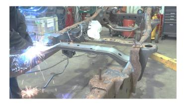
Then, hold the two remaining plates up to each end of your crossmember on the outer side of your frame rail, followed by tacking them into place. Then, weld the plates on fully. Weld 100% around all edges.
