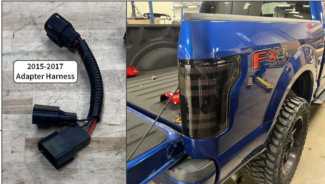
**2015-2017 Model Year Only:** Plug in the included adapter harness into the corresponding vehicle tail light connector.
