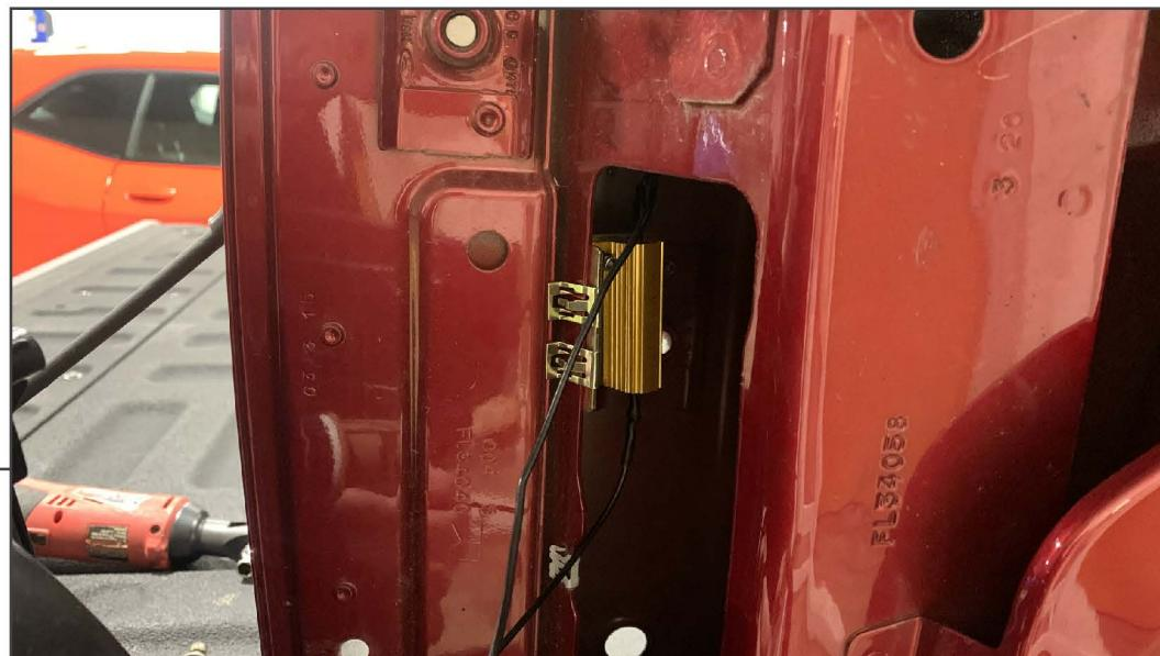
Using (2) vampire clips, secure the resistor bracket to the inside of the tail light area of the vehicle. Ensure the resistor is placed away from the tail light wiring connector(s).
