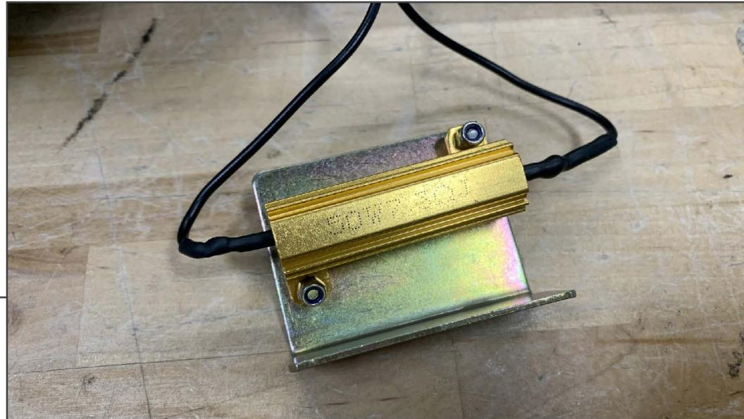
Secure the resistor to the resistor bracket using (2) M4 bolts and (2) M4 nuts. Tighten the hardware until secure.
