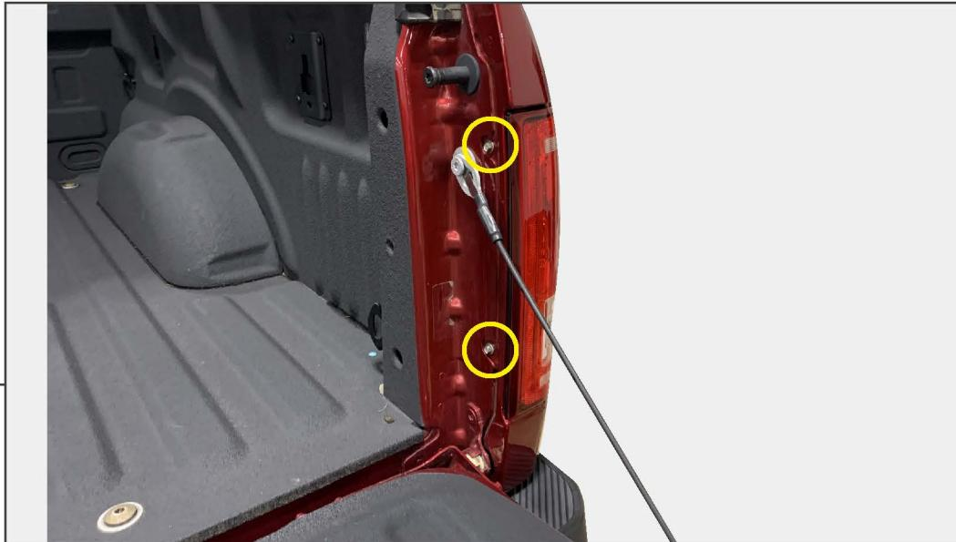
Lower the vehicle tailgate and remove (2) 8mm bolts from the tail light assembly.
