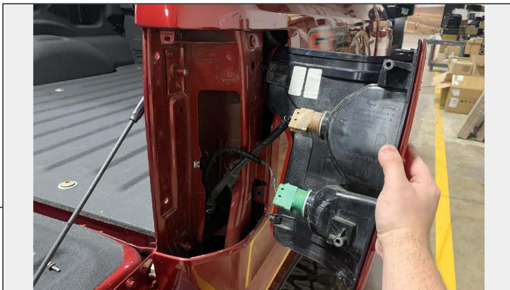
Firmly pull the tail light rear-wards to dislodge the (2) alignment pins in the vehicle bed.
