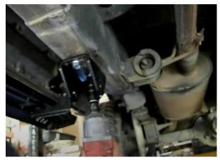
8.Attach the traction bar to the frame bracket using the supplied M14 -100mm bolt and hardware.
