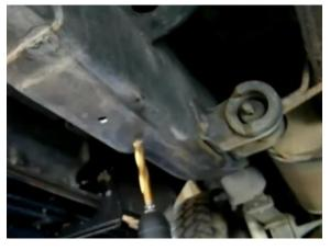
6.Insert the M12 flag nut into the frame from the side and align it with the drilled holes. If alignment is difficult, you can use a 9/16" drill bit to enlarge the hole. A Larger hole size allows for easier adjustment.
