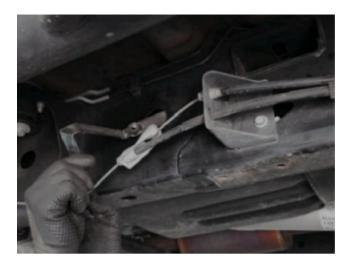
7.Mount the Frame Bracket using the M12
