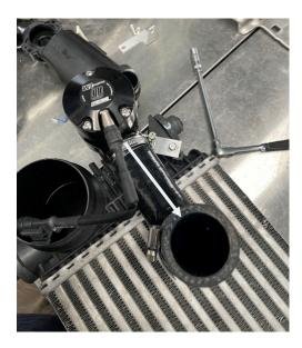
The alignment of the diverter valve is important. The diverter valve can screw in with two directions. The recirculation port must face towards the intercooler as pictured above.
