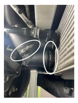
The two 7mm hose clamps must be correctly clamped.
