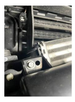
The chamber pictured below can be removed, the chamber is simply rotated anticlockwise and it will uncouple from the intercooler.
