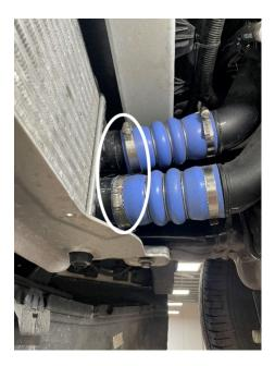
The recirculation pipe must be fitted ensuring the connector clips and locks into place, at this point we should tighten up any loose hose clamp to ensure that we have correct orientation of the recirculation pipe.
