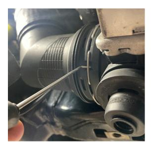
The Turbo feed charge pipe also need to be removed. These are also held on with 7mm hose clamps.
