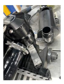
The mount that holds the valve comes in two options. The most suitable one needs to be used. The Smaller right angled one pictured is for the small version intercooler. We must use a M3 Allen key to attach to the diverter valve.
