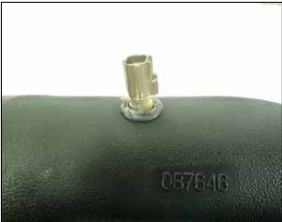
14. Remove the O-ring from the IAT sensor and then install the sensor into the K&N intake tube using the provided grommet.
