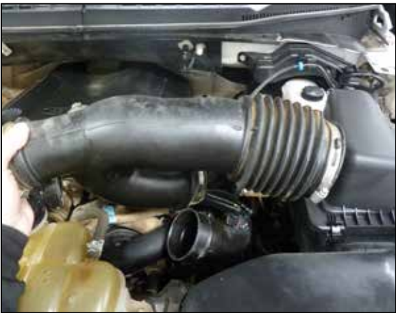
5. Remove the factory intake tube from the vehicle.
