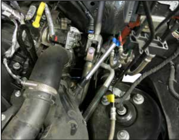
8. Disconnect the CCV connection shown on the drivers side turbo inlet tube.
