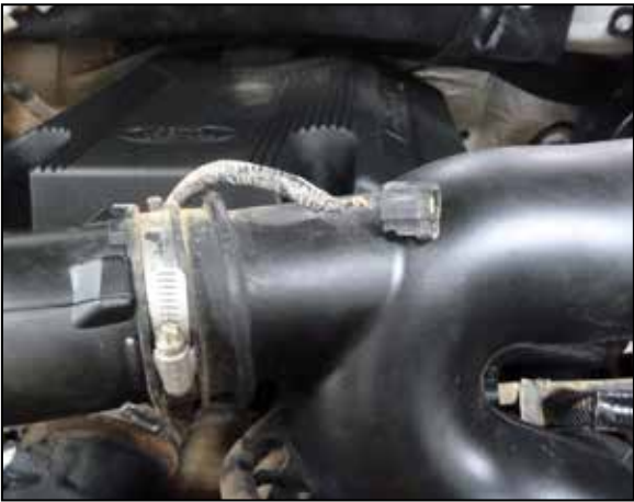
4. Disconnect the IAT sensor electrical connection from the factory tube. Unhook the wiring harness from its mounts.
