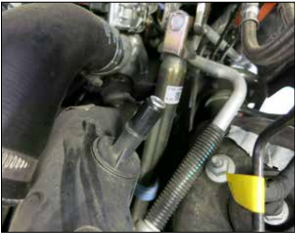
10. Once the insert is slid completely into the fitting reconnect the CCV connection.
