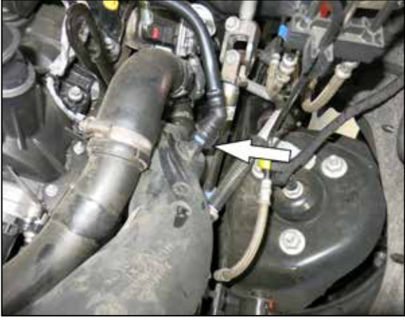
8. On 2021 and earlier 3.5L Ecoboost vehicles, Disconnect the CCV connection shown on the drivers side turbo inlet tube. On later 2022 and later model vehicles skip to step #11.
