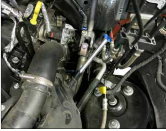
8. On 2021 and earlier 3.5L Ecoboost vehicles, Disconnect the CCV connection shown on the drivers side turbo inlet tube. On later 2022 and later model vehicles skip to step #11.
