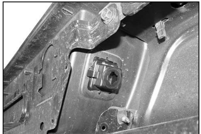
(Fig 6) Disassemble bumper to remove license plate lights, trailer plug, sensors and wiring harness from bumper as equipped
