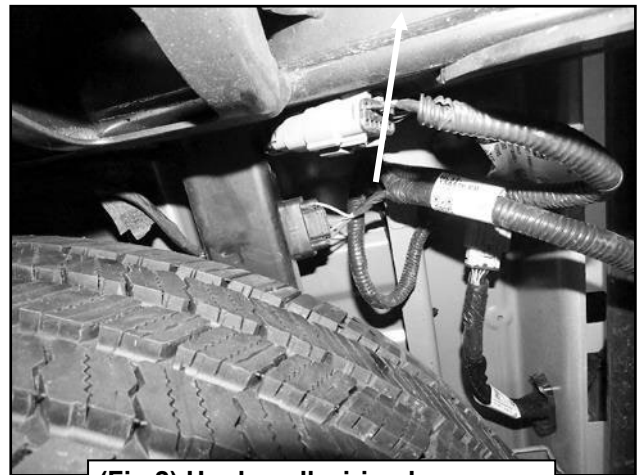
(Fig 2) Unplug all wiring harnesses leading to bumper
