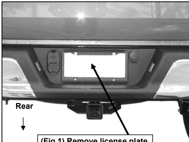
(Fig 1) Remove license plate
