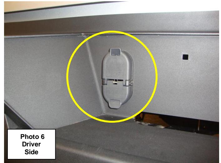
**Step-12** Reconnect the factory bumper wiring harness to the sensors and to the vehicle wiring harness.
