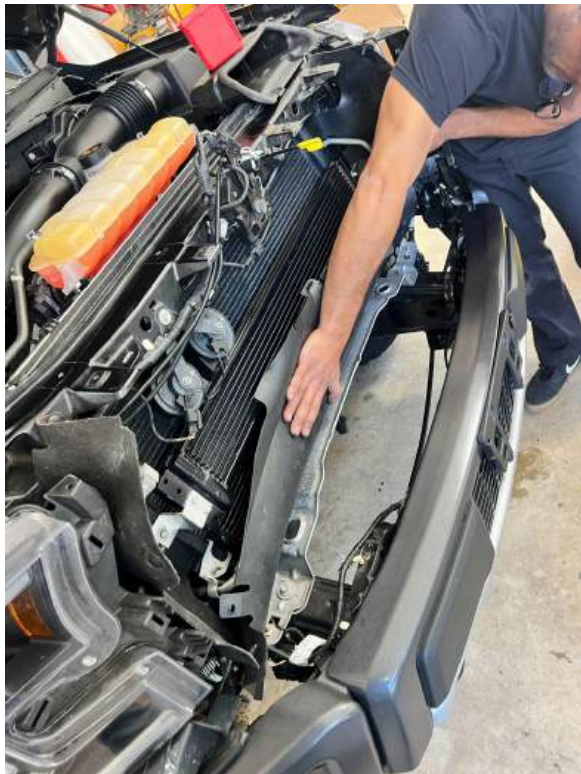
16b. Remove Metal Bracket from upper intercooler mount.
