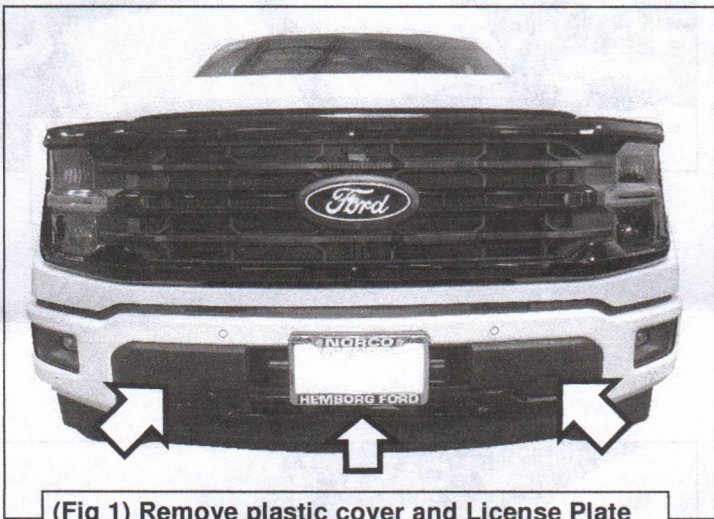
(Fig 1) Remove plastic cover and License Plate Bracket from Front Bumper.
