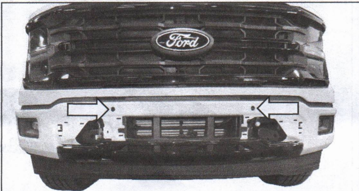
(Fig 5) Spread tabs on plastic sleeves and remove parking sensor (Front Bumper removed for illustrative purpose only)
