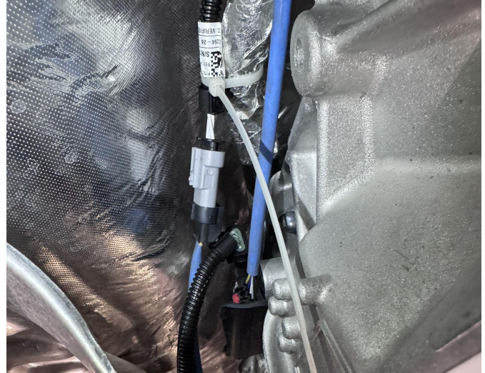
Detail 18: O 2 Extension is run over top of the transmission and ziptied into place.
