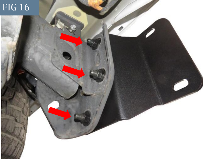
(Fig 16) Attach passenger/right Mounting Bracket to vehicle with OEM bolt plate and hardware
