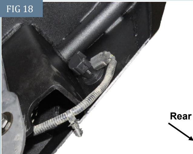
(Fig 18) Attach wire connectors to parking sensors
