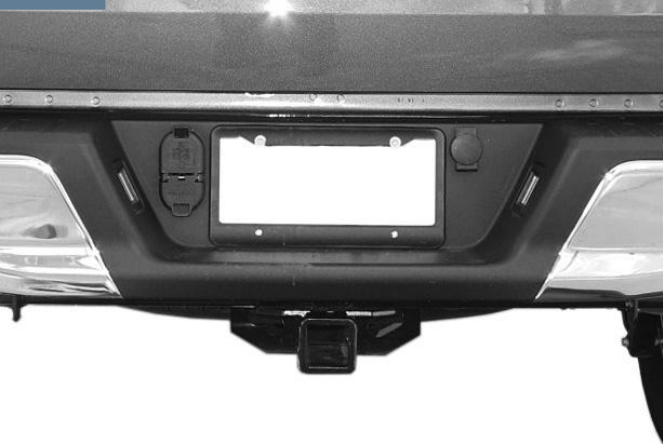
(Fig 1) Unplug and remove 7-wire trailer plug
