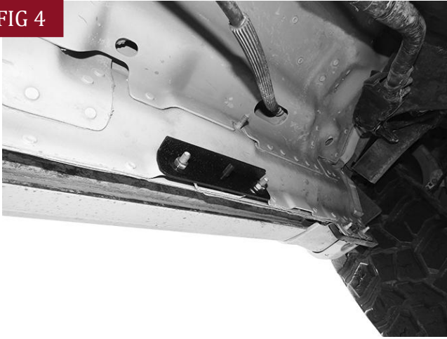
(Fig 4) Example of the Support Bracket (#1) attached to the threaded studs
