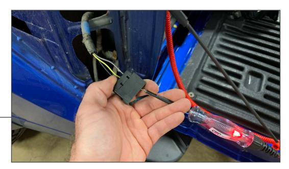
Remove the tail light to access the factory wiring. With the key on and ENGINE OFF, apply the emergency brake and have a helper step on the brakes. Using a test light or multimeter, locate the 12volt power supply for the factory brake light. Confirm the wire only has power when the brakes are applied. Using the supplied scotch lock connector, connect the Brown wire from the tailgate light to the factory brake light wiring.
