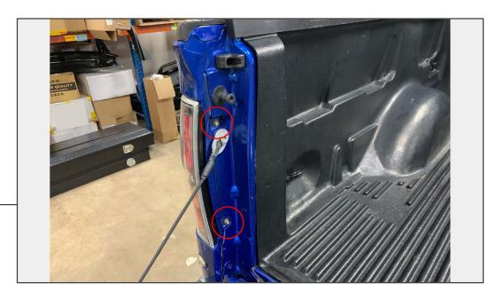
Additional wiring will require access to the factory tail light wiring. Begin by removing the fasteners that hold the tail light to the vehicle.
