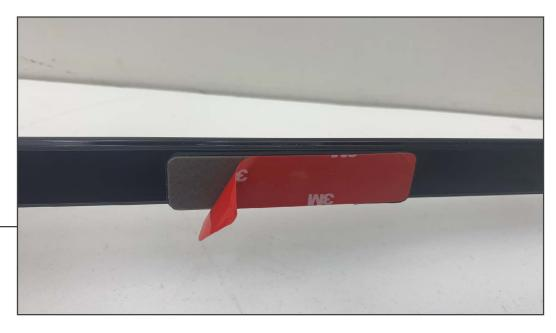
Test fit the tailgate light bar prior to removing the tape back. The wiring has to exit the tailgate light bar on the driver side of the vehicle. Once you are comfortable with how the tailgate light bar fits, remove the tape backing and install the tailgate light bar.
