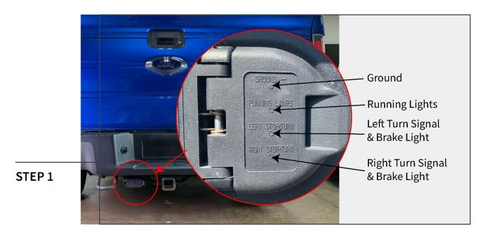
Begin the installation by locating the factory 4-Pin tailer plug. Using a test light or multi-meter, test the trailer plug for all functionality (turn signals, running lights, and brake lights). If the plug isn't getting power, reference your owners manual to locate and test the trailer plug fuse.
